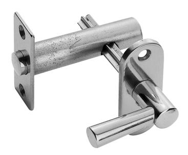
Security bolt with a cylindrical turn lever on a radius backplate. By rotating the small turn handle it engages the teeth on the bolt and slides it out smoothly from its housing into the opposing plate on the door frame, thereby locking the door. Reversing direction of handle retracts it back into position. Provides additional security, convenient and easy to use.
