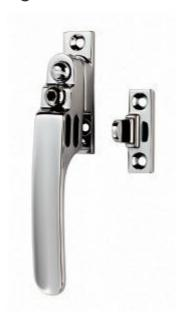
Heavy duty Victorian locking casement fastener with night vent option. Locking function, fully reversible so can used on Left hung or Right hung windows. Features a two-position night vent. The arm has two slots in the side, if the handle is moved to engage either of these slots in the staple it allows the window to be marginally open allowing air circulation but retaining full security.
