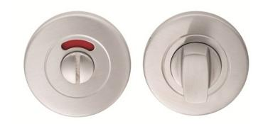
Standard Turn and Release with a vacant/engaged Indicator. Concealed fix press on rose. Stylish bathroom turn and release, thumb turn on one side and an emergency release slot on the other. Part of the Steelwork range in Grade 304 Stainless Steel and will match all of the Steelworx levers.
