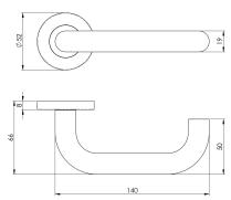
Lever on concealed fix press on round rose. Safety Lever, a 19mm round bar return to door lever. Ideal for public/office doors where a more ergonomic operation is a necessary requirement. Part of the Steelworx range in grade 201 Stainless Steel.
