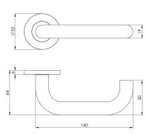
NERA Lever on concealed fix press on sprung round rose. Safety Lever, a 19mm round bar return to door lever. Ideal for public/office doors where a more ergonomic operation is a necessary requirement. Certified to BS8300 to meet the needs of disabled people.
