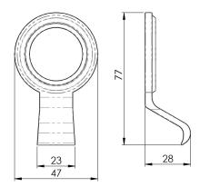
A highly popular latch pull. Fitting around a Yale type cylinder used on a night latch, It is used to pull the door closed from the outside. The lower part of the pull projects further forward than standard pulls thus providing ample finger purchase.
