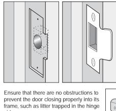
Position the strike plate on the door frame so that it lines up with the flat of the latch bolt, NOT THE PLUNGER.
