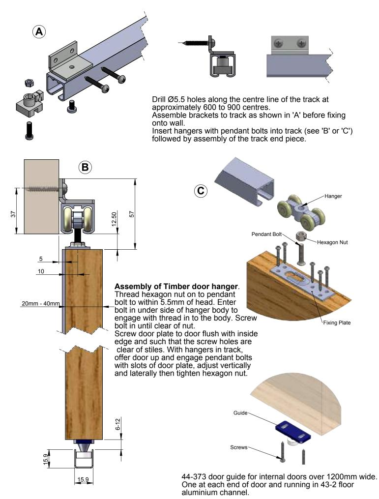
CAUTION: Do not wind the Pendant Bolt all the way past the top of the Hanger, as this will stop the system from working properly
