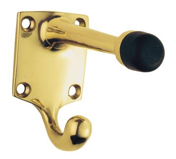
One piece hat and coat hook with rubber buffered end to protect the door. The hat hook with the buffer tip extends straight out and the coat hook is suspended below the base plate which has 4 anchor points for a secure fixing.
