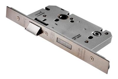
Easi-T Din Bathroom Lock 60mm. Square and Radius options. The Latch bolt has the Easi-T reverse function to save undoing the case so it can be reversed in seconds. Certified to BS EN 12209.
