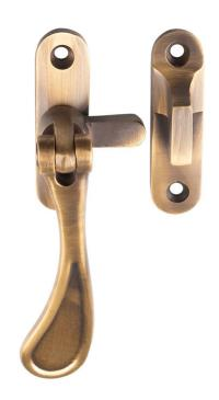
A plain spoon ended pivot-reversing non-locking casement fastener, one of the most commonly used fasteners for traditional timber windows. It operates with either a mortice or hook plate and is reversible. Not suitable for use on weather stripped windows. Comes with a 10 year mechanical guarantee.
