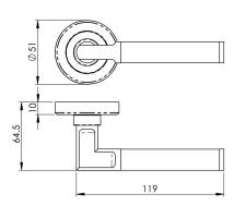
Lever on a chamfered edge concealed fix screw on round rose. A round bar sectional lever with a flattened mitred corner. The lever features a dual finish emphasising the sectional components which highlights the modernistic influence. Part of the Serozzetta Residential range.
