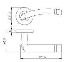
Lever on a concealed fix press on round rose. The Cuarenta lever on rose features etched rings detailed at the end with a gentle curved handle which fits nicely into the palm of the hand. Comes with a 10 year mechanical guarantee and is Fire door rated. Suitable for domestic and commercial use.
