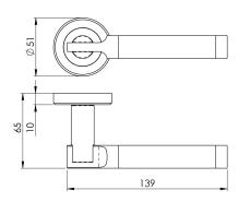
Lever on a concealed fix 2 part screw on round rose. A stylish round bar lever with a dual finish. The chamfered edge concealed fix rose reflects the attention to detail in this range. Comes with a 10 year mechanical guarantee and is Fire door rated.
