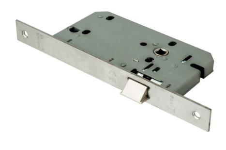
Contract Din Latch, 55mm. Square or Radius option. The Latch bolt has the Easi-T reverse function to save undoing the case so it can be reversed in seconds. Certified to BS EN 12209.
