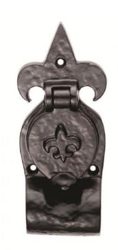
Black Antique rim cylinder latch pull with a fleur-de-lys pattern at the top and on the key access cover shield. Fitting around a Yale type cylinder used on a nightlatch, it is used to pull the door closed from the outside. The lower part of the pull projects forward providing ample finger purchase. The cover shield is hinged at the top and when lifted reveals the lock (supplied separately).
