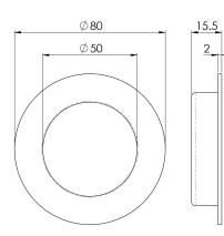
78mm Dia. circular shaped low profile flush pull which is used mainly on sliding doors. The main cup is recessed back into the door to leave a flush appearance. For use on doors, wardrobes or cupboards.
