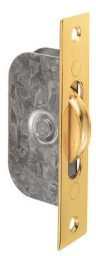
Sash window axle pulley with square brass forend and a brass wheel. A range of sturdy axle pulleys for sliding sash windows. Sash window axle pulleys are used in traditional rise and fall sash windows to carry the cord attached to the window counter balance sash weight. Typically you will find four in any sash window, two for the top sash and two for the bottom sash.
