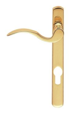
Fashionable, traditional style scroll lever on a Euro lock narrow backplate. It has a Euro profile keyhole and operates a multipoint lock. This handle is handed depending on which side the door is hinged and whether inward or outward opening. The right or left option will need to be specified when ordering.
