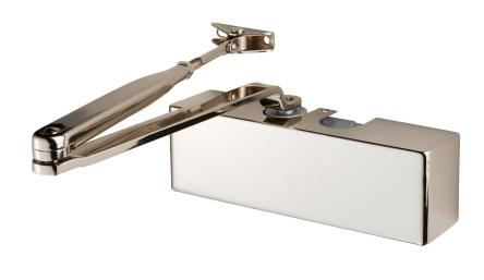
CDG420 is a template adjustable overhead door closer, EN 2 " 4, which is suitable for inward or outward opening doors up to 80kg in weight, and/or 1100mm wide. It has been successfully tested in all installation applications to BS EN1154:1996, and covered by CE and Certifire accreditations. Suitable for use on timber fire doors, up to 120 minute rating. Includes a cover and Fig6 bracket as standard.
