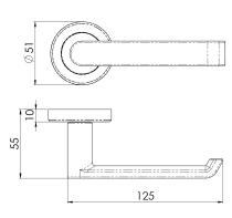
Lever on a concealed fix 2 part screw on round rose. A favoured design for the commercial environment is the Concept lever. The bold face of the lever and return to door feature gives visual impact along with safety. The chamfered edge concealed fix rose reflects the attention to detail in this range.
