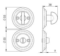
Bathroom turn and release set to compliment the Delamain door knob range. Use of a separate deadbolt is required). Comes with a 10 year mechanical guarantee. Available in different finishes.
