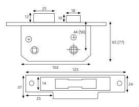
All dimensions are in mm and are nominal. Numbers in brackets relate to 3" version of lock. Diagram illustrates product in locked position. ERA reserves the right to change specification without notice It is the responsibility of the door manufacturer to ensure that the finished product meets any required safety and performance specification.
