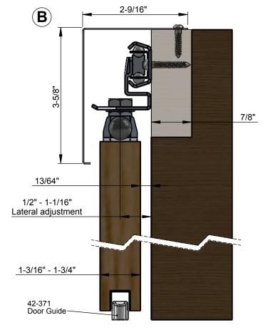
Stand door in closed position on 1/4" packing. Position track by aligning pendant bolts with slots in hangers and arranging for the inner bar to stop 1/4" clear of peg in end of track. On no account must this peg be used as a stop. Track must be perfectly level on track plate 'E' with top edge of track 2-5/8" above the final position of the top of door. Use bradawl for screw holes in order to avoid wood chips in track - fig. C. Fix with seven No. 8 x 1" Csk head screws.
