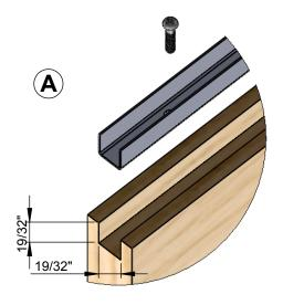
Groove bottom of door to suit 42-1 channel size19/32 "  $\times$  19/32") cut channel to suit door. Fix with No. 6  $\times$  3/4" countersunk woodscrews- fig. A.
