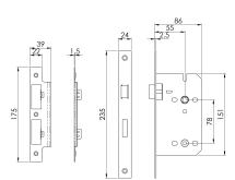
Contract Din Bathroom Lock 55mm. Square and Radius options. The Latch bolt has the Easi-T reverse function to save undoing the case so it can be reversed in seconds. Certified to BS EN 12209.
