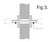
Check against the door to make sure that the length of spindle will fit through the door and locate with the opposite lever . "If fitting levers to doors thicker than 44mm A longer 120mm spindle (ALS1002H) will be required ."
